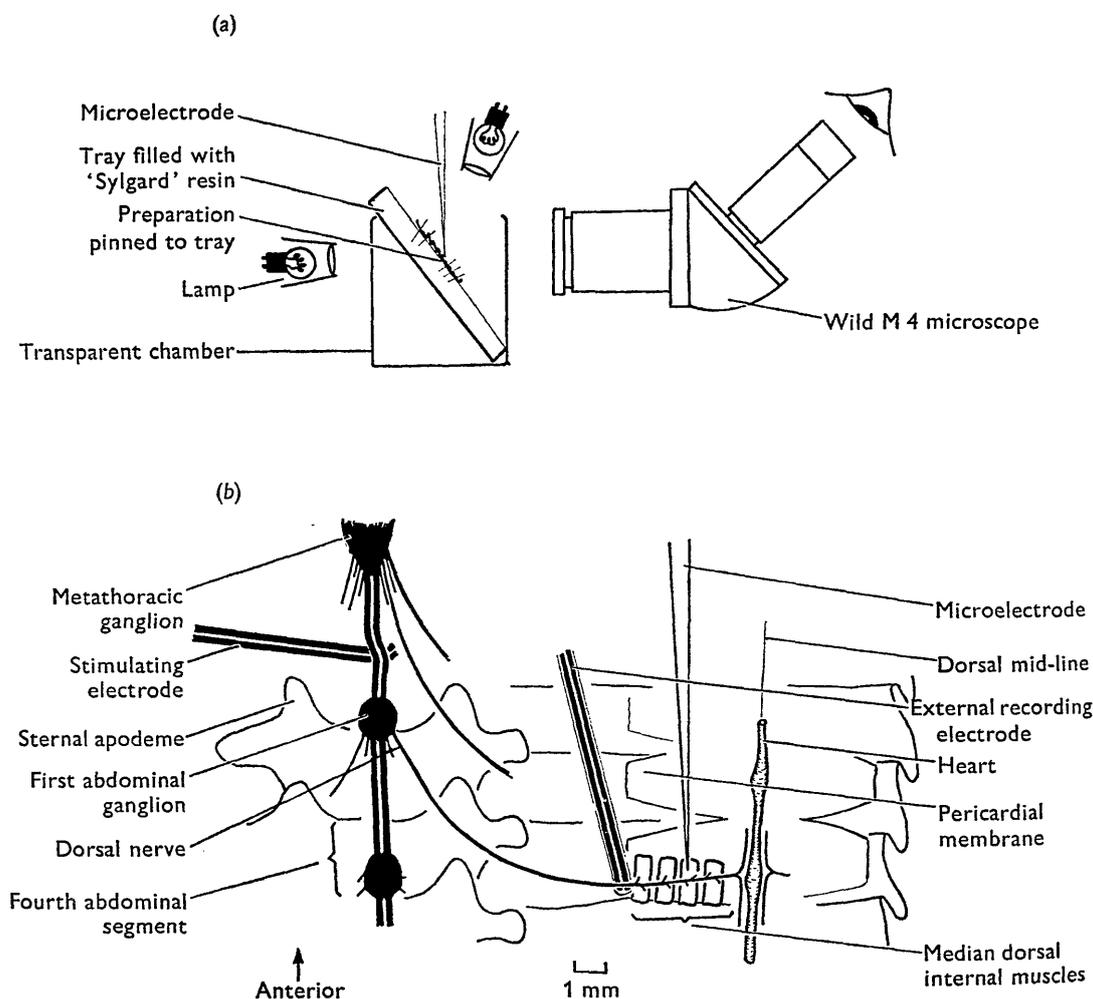
Fig. 1. (a) Arrangement of the preparation for recording. The preparation was viewed from the side to monitor the advance of the electrode precisely, and the muscle fibres were impaled at a shallow angle to their length. (b) Diagram of the abdominal segments two, three and four to show the position of the microelectrode, external bipolar electrode and stimulating electrode.
