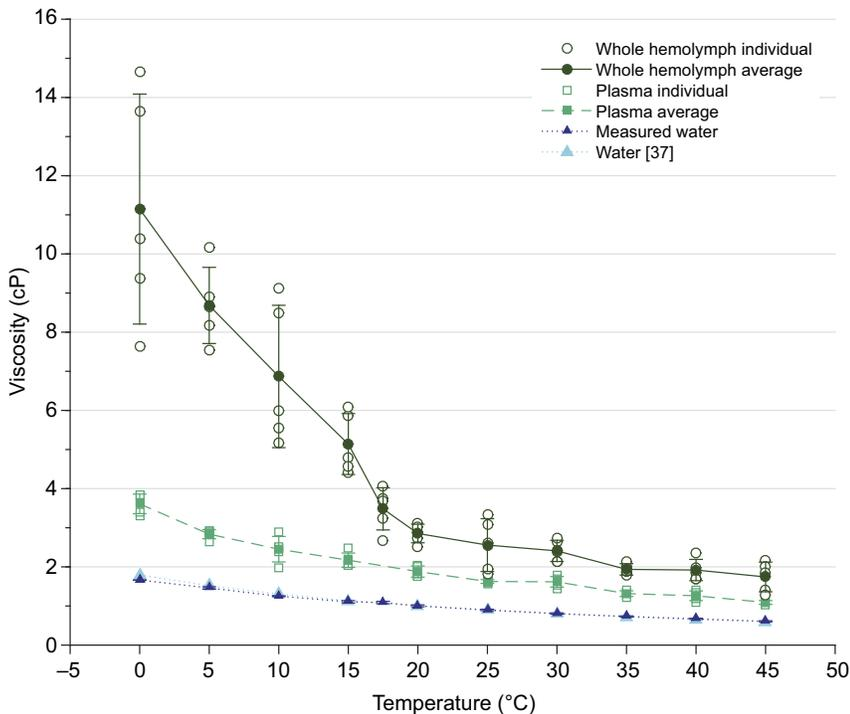
**Fig. 2. Temperature dependence of viscosity for whole hemolymph and plasma of *Manduca sexta* larvae.** Known values of water (from Kestin et al., 1978) are shown for comparison. Filled points represent the mean value for each temperature, with the individual trials shown as non-filled points. Error bars represent standard deviation of the mean. The quantitative fits for each trend are provided in Eqns 1 and 2.
