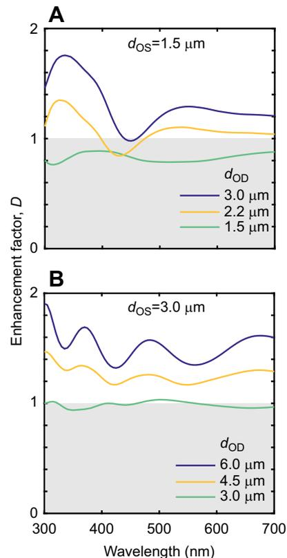
**Fig. 4. Simulated enhancement factors for increasing sizes of oil droplet.**  $l_{OS}=30\ \mu\text{m}$  and  $n_{OD}=1.5$ . Grey regions indicate oil droplets resulting in loss of light. Larger oil droplets result in greater enhancement factors. Wider outer segments and larger oil droplets give larger enhancement factors.
