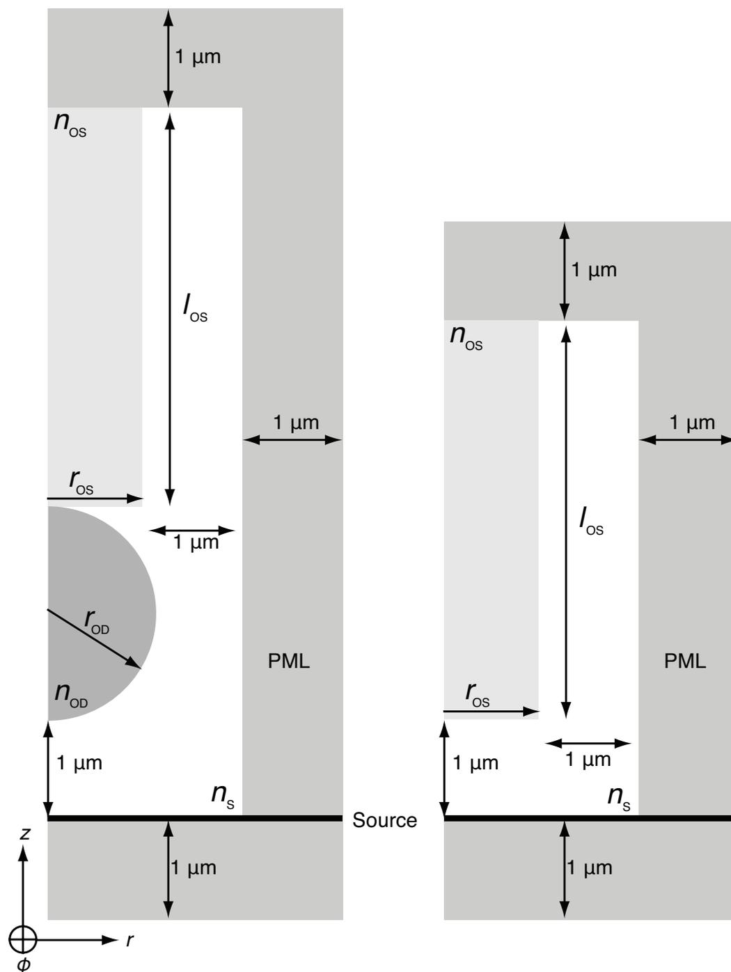
**Fig S1: Example schematics of the simulation environment.** Thick black line indicates the plane wave source. Calculations are performed in cylindrical polar coordinates  $(r, \phi, z)$ .  $\phi$ -direction is normal to the plane of the page here. Simulation is surrounded on three sides with perfectly-matched layers (PML) which prevent numerical reflections from the sides of the simulation environment (Oskooi et al. 2010).
