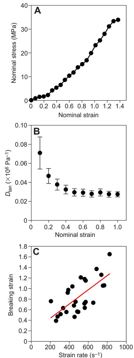
**Fig. 6. Results of the high strain rate tensile tests.** (A) A representative stress–strain curve. The strain rate in this test was  $688 \text{ s}^{-1}$ . (B) Average compliance ( $D_{\text{tan}}$ , tangential compliance) as a function of strain; the error bars are s.e.m. (C) Breaking strain is positively correlated with strain rate.
