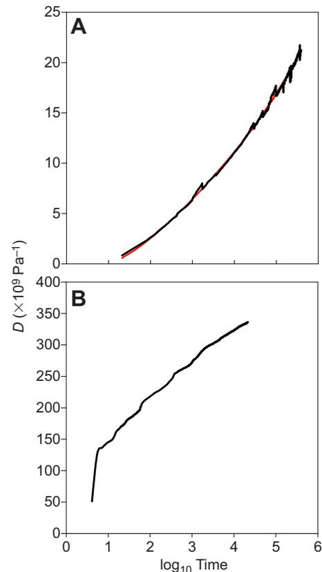
**Fig. 9. Average creep behavior of genicular material in tension and shear.** (A) In tension, different samples survived for different periods, leading to the ragged jumps in compliance ( $D$ ) as the number of tests included in the average decreased as time increased. Red line is a fit to the data. (B) Creep in shear. Time was measured in s.
