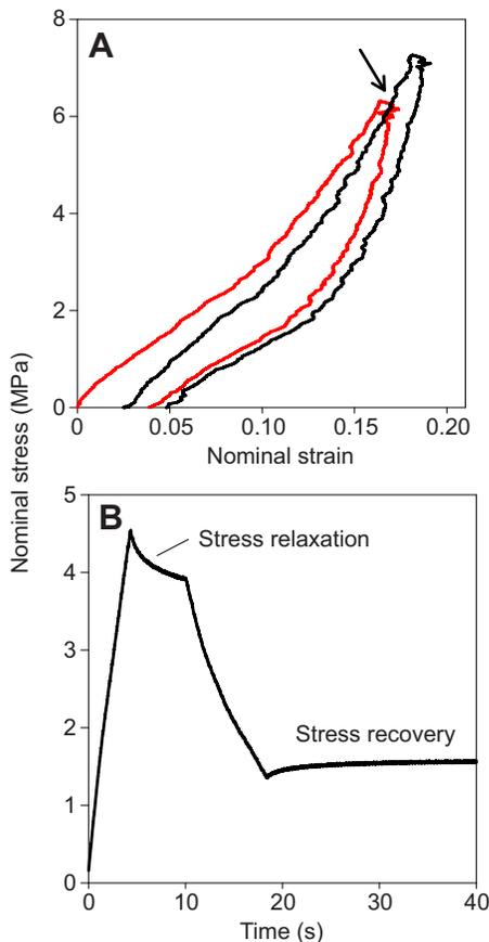
**Fig. 7. Results from the cyclic tensile tests.** (A) Representative results from the initial two cycles of strain. The red line is the first cycle, the black line the second cycle. Note that the stress due to incremental strain in the second cycle takes up where the first cycle left off (arrow). (B) A test showing stress relaxation when the moving head is stopped while stress is increasing, and stress recovery when the head is subsequently stopped as stress decreases.
