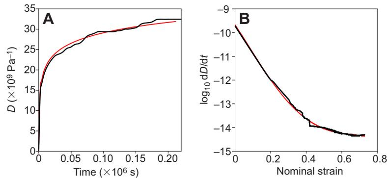
**Fig. 4. Creep and compliance in *C. cheilosporioides'* genicula.** (A) A representative record of tensile creep. The red line is a logarithmic fit to the data:  $y=3.703\ln(x)+37.648$  ( $r^2=0.986$ ), where  $x$  is time ( $\times 10^6$  s) and  $y$  is compliance ( $D, \times 10^9 \text{ Pa}^{-1}$ ). (B) Compliance expressed as a function of strain rather than time. The red line is a polynomial fit to the data:  $y=-27.813x^4+40.85x^3-8.215x^2-11.372x-9.6624$  ( $r^2=0.981$ ).
