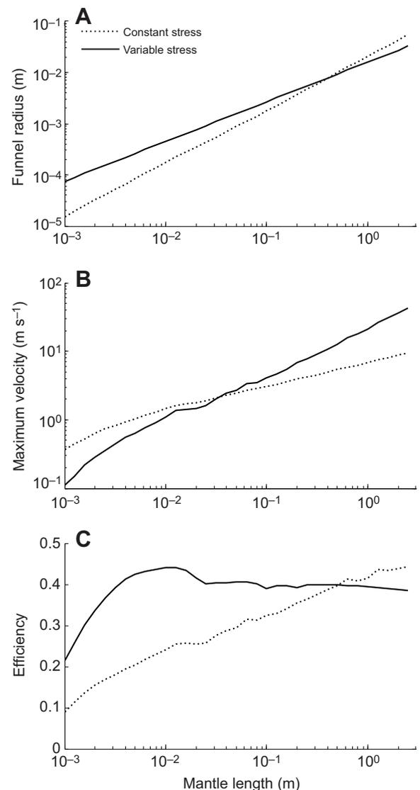
**Fig. 5.** Size-dependent variation in jetting when variables are set by regressions with a dynamically varying aperture, allowing stress to vary (solid lines), compared with when funnel radius is controlled to maintain a constant stress of  $2.5 \times 10^5 \text{ N m}^{-2}$  (dotted lines). (A) Size-dependent variation in funnel radius. (B,C) Theoretical results of using this radius for maximal squid velocity at the peak of a single jet (B) and hydrodynamic efficiency (C).
