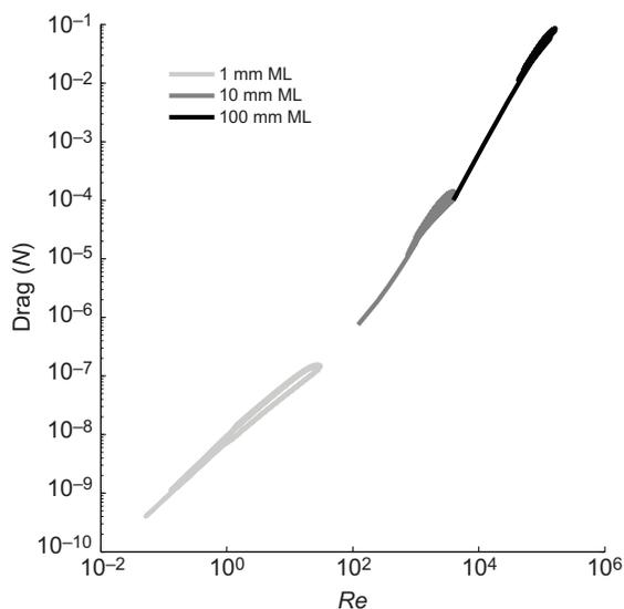
**Fig. 9. Drag as a function of Reynolds number for three sizes of squid.** Data for 10 cycles of contraction and refilling are plotted for each squid (1, 10 and 100 mm ML); loops emerge because drag depends on both  $Re$  and squid velocity.
