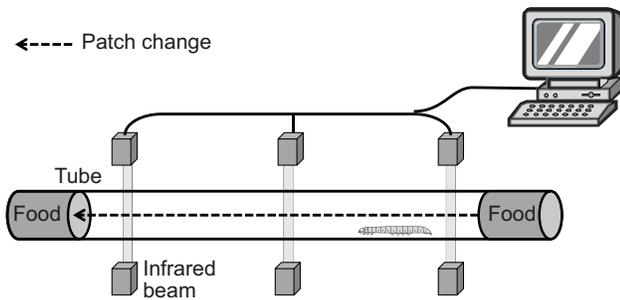
**Fig. 3. Schematic illustration of one tubular unit of the actimeter, used to automatically record individual larval foraging behaviour.**
