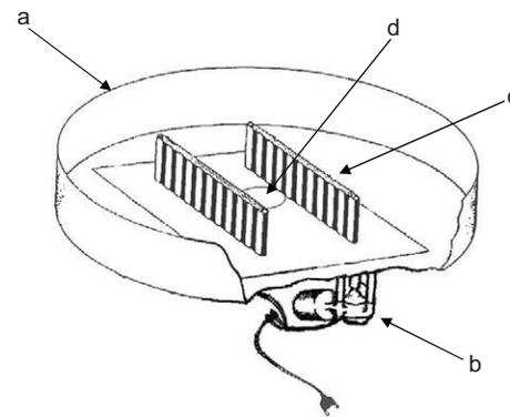
**Fig. 2. Device used to produce an artificial optic flow (modified from Ugolini, 1987).** (a) Screen for the natural landscape; (b) electric motor for moving the walls with the black and white stripes; (c) walls with black and white vertical stripes used for the artificial optic flow, (only two of the four walls are represented). During the experiments, the Plexiglas bowl with sandhoppers was placed between the walls, on the transparent plate (d).
