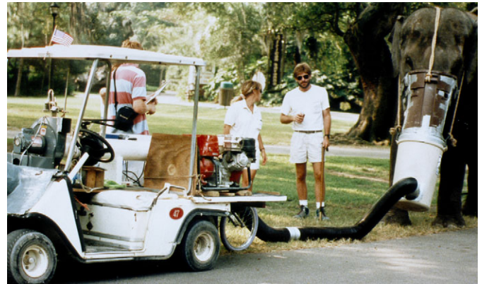
Fig. 1. Open-system measurement of resting oxygen consumption in a female Asian elephant prior to exercise at Audubon Zoo, New Orleans, LA, USA.
