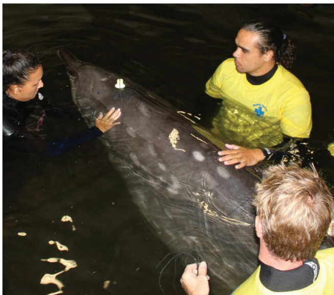
Fig. 3. Experimental setup; the active suction cup is visible behind the blow hole of the beaked whale. The animal was lightly restrained during hearing measurements.
