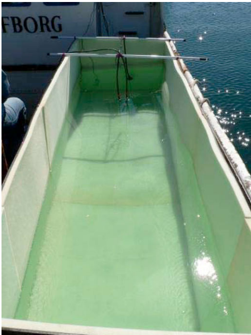
Fig. 3. Experimental plastic tank lined with open cell foam.
