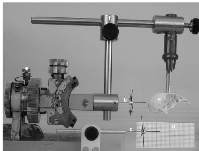
Fig. 1. Rotating device used to take photographs of a rotating skull. A, skull; b, fixed XYZ axes; c, rotating XYZ axes; d, millimeter paper; e, pin to set the angle; f, adjustable tubes.
