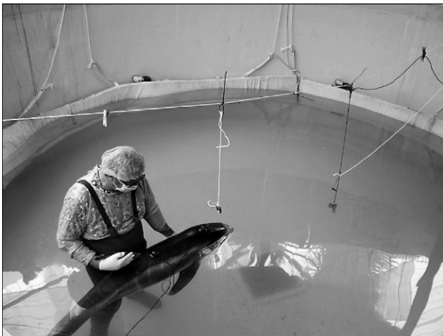
Fig. 2. Experimental design in the rehabilitation pool. The infant Risso's dolphin was held by the experimenter in its position 0.5 m from the center of the pool and 1 m from the suspended hydrophone.
