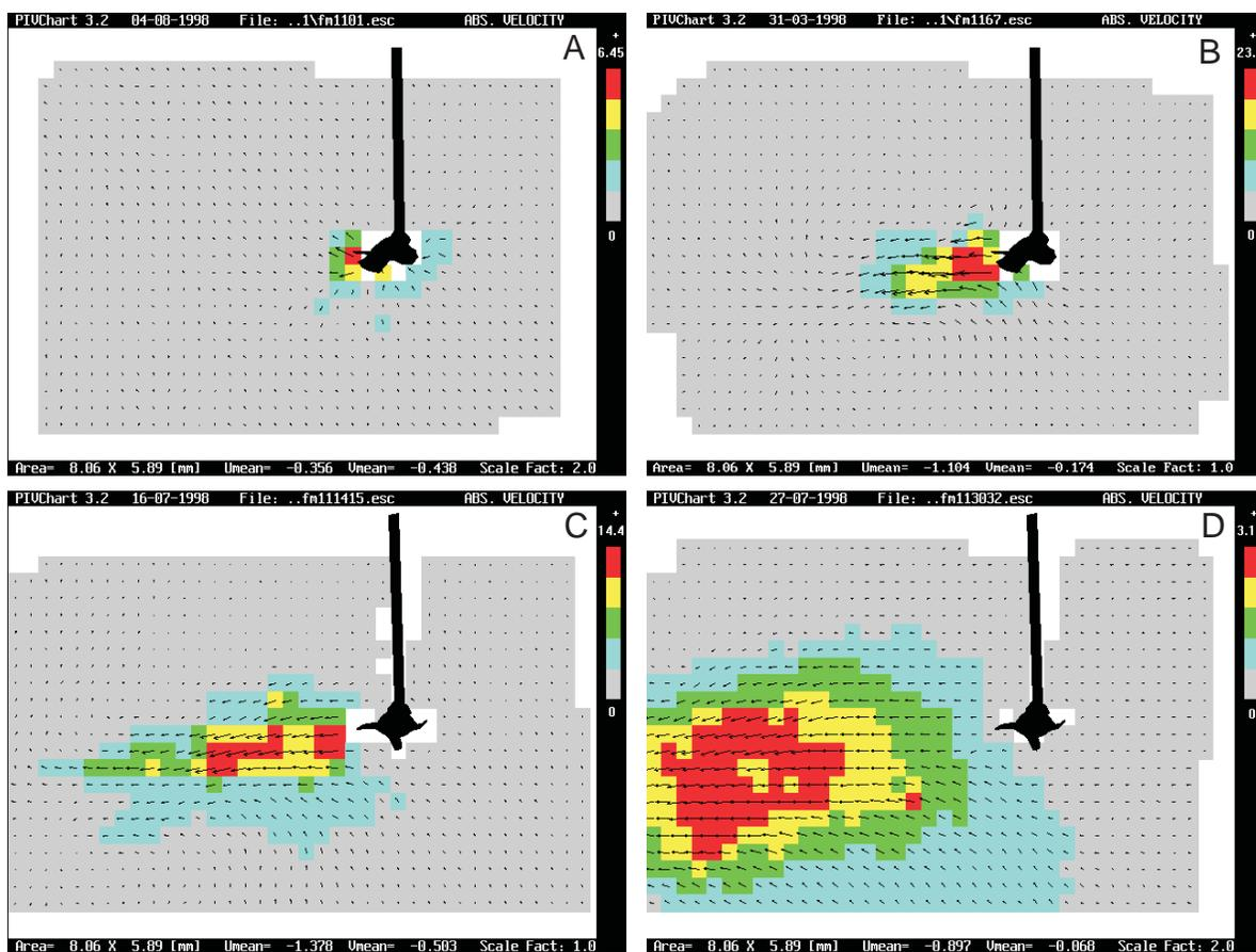
Fig. 6. Sequence of velocity distribution plots around an escaping copepod. (A)  $t=0$  s, (B)  $t=0.08$  s, (C)  $t=0.28$  s and (D)  $t=0.5$  s. Note that colour coding is a relative scale, i.e. different for each individual flow field.
