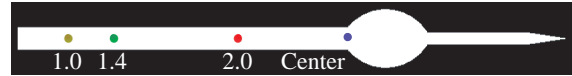
Fig. 9. Centered particles are transported more efficiently. Four simulations were run in which we measured the final position after a single cycle of a single particle placed at the mouth at time zero. The brown particle was assumed to move at mean fluid velocity as in previous simulations. The green and red particles move at 1.4 and 2.0 times mean fluid velocity, respectively, and the blue particle moves at the calculated velocity of the fluid at the center of the lumen, which varies from 2.2 to 3.5 times mean velocity depending on how open the lumen is at a particular moment. See text for further explanation.
