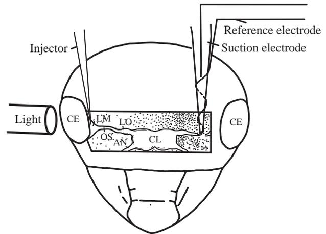
Fig. 1. The arrangement used to record neural activity from the optic stalk brain efferents. Neural activity was recorded from the separated optic stalk using a suction electrode. Light stimulation and injection of chemicals were performed on the contralateral side. AN, antennal nerve; CE, compound eye; CL, cerebral lobe; LM, lamina medulla complex; LO, lobulla; OS, optic stalk.
