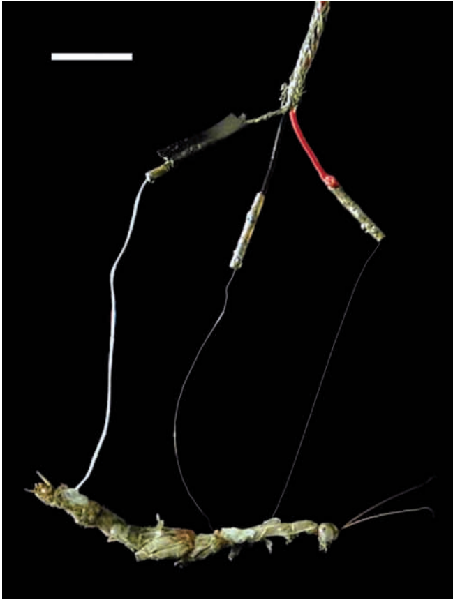
Fig. 1. The implanted electrode arrangement in the hanging tethered mantis preparation. Scale bar, 10 mm. The right-hand wire holds the clip electrode and the connective, the middle wire holds the indifferent lead and the left-hand wire stabilizes the mantis in a 'flight-like' posture.
