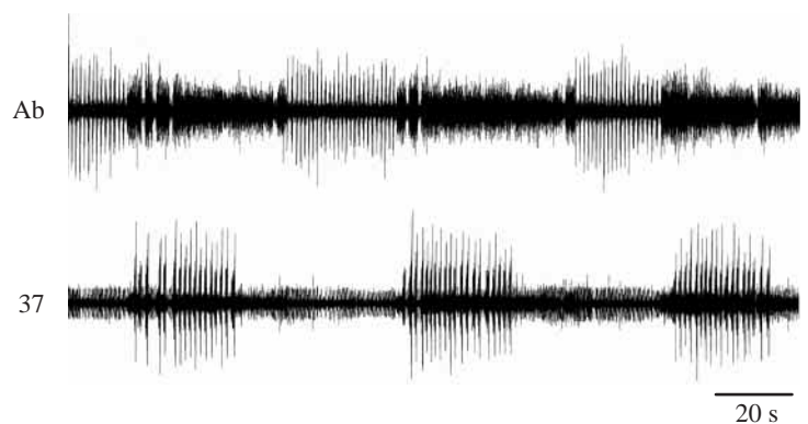
Fig. 6. Alternation between bouts of ventilation rhythm and frontal ganglion (FG) rhythm can be seen during air swallowing in recordings from an abdominal muscle (Ab) and a foregut dilator muscle (37).
