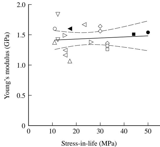
Fig. 4. Young's modulus for different tendons. No correlation with stress-in-life is observed:  $r^2=1.1 \times 10^{-2}$ ,  $P=0.69$ ,  $N=18$ . Symbols are as in Fig. 1. The open symbols are data from the present study. The filled symbols are from Ker et al. (1986). Linear regression and 95% confidence limits are shown.
