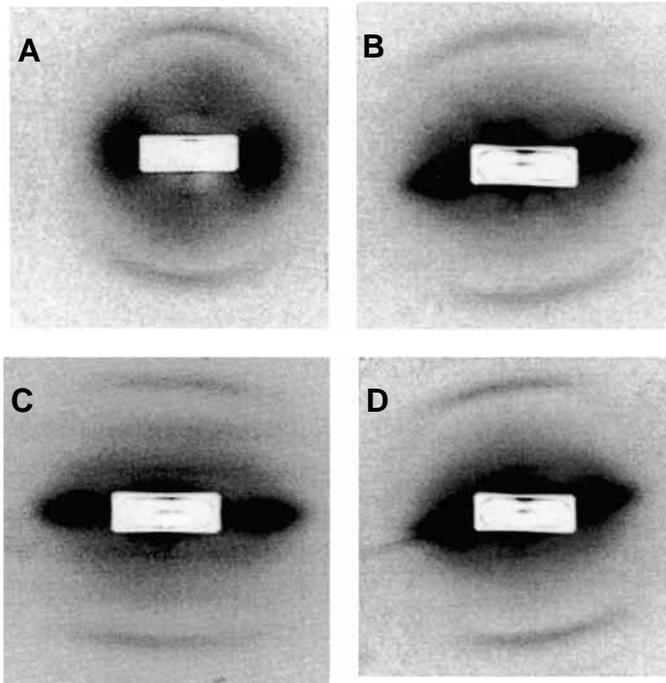
Fig. 1. Small-angle X-ray diffraction patterns from two specimens (A,B) showing different degrees of structural ordering at initial length. Extension by approximately 50% of the specimen in A results in increased ordering (C), but similar extension of the specimen in B results in little change (D).
