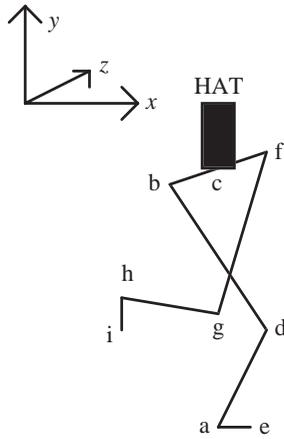
Fig. 1. Sketch of the model indicating joints and segments. The positive  $x$  axis points forward; the  $y$  axis points cephalic; the  $z$  axis points to the left. HAT, head, arm and trunk. Joints: e/i, ball of foot; a/h, ankle; d/g, knee; b/f, acetabulum; c, center of pelvis. Links: ae/hi, foot; ad/gh, calf; db/fg, thigh; bc/cf, half of pelvis.
