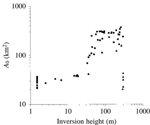
Fig. 2. Zero-wind,  $-67$  dB calling area ( $A_0$ ) as a function of inversion height, for 65 tethersonde runs. Surface inversions and non-inversion profiles are shown by circles, elevated inversions by triangles.
