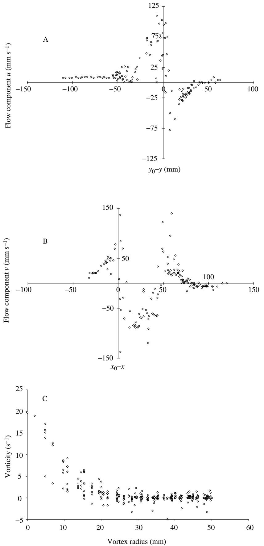
Fig. 6. Velocity and vorticity profiles of vortices from Fig. 5B. The transect runs through the core of the vortex; the width of the transect is 10% of the vortex ring diameter. (A)  $u$  velocity profiles through vortex 1 from Fig. 5B. (B)  $v$  velocity profile through the vortex system formed by vortices 1 and 2 from Fig. 5B. (C) Vorticity  $\omega$  profile of vortex 1 from Fig. 5B.
