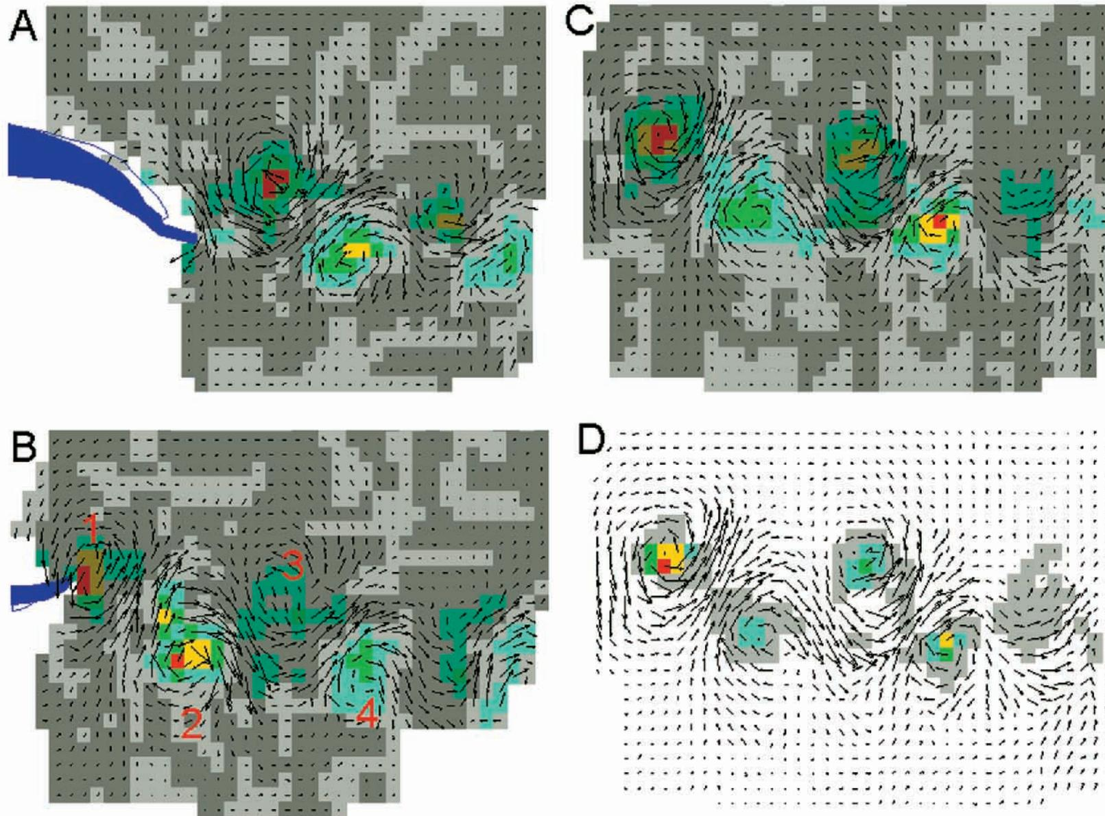
Fig. 5. The wake of a continuously swimming mullet (field of view  $0.195\text{ m}\times 0.175\text{ m}$ ); vector information was obtained by combining PIV and PTV data. The arrows represent the flow velocity in  $\text{mm s}^{-1}$ ; the colour code represents vorticity in A–C, with bright shades indicating clockwise vorticity and dark shades indicating counter-clockwise vorticity; the
