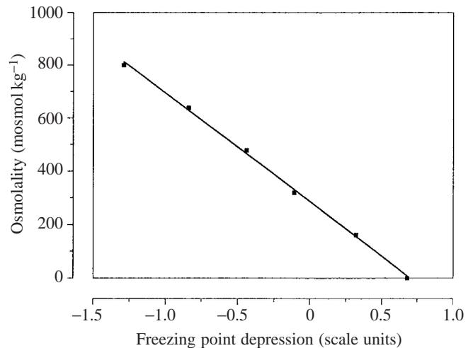
Fig. 4. Example of a calibration curve for the nanolitre osmometer shown in Fig. 3. Distilled water or solutions of NaCl of varying osmolality were used, and their freezing points determined.
