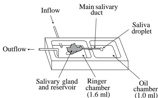
Fig. 1. Schematic representation of the perfusion chamber used for the collection of saliva from isolated cockroach salivary glands.
