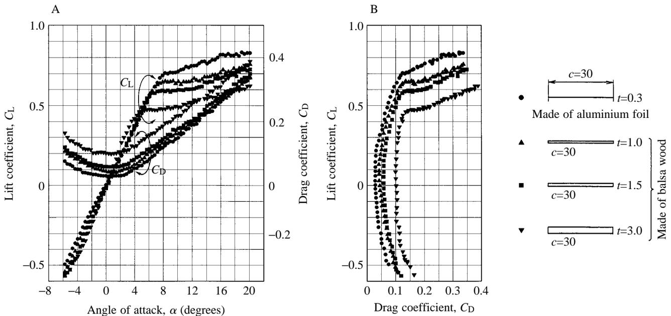
Fig. 6. Effects of the thickness of a flat plate on its aerodynamic characteristics. Each symbol refers to a different model, the shape of which is shown in the panel on the right of the figure;  $t$ , thickness,  $c$ , chord length. All measurements are given in millimetres. (A)  $C_L$  and  $C_D$  versus  $\alpha$ . (B) Polar curve.
