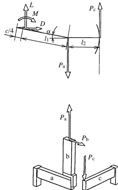
Fig. 3. Forces and moment derived for the load cells contained in the balance system. Load cells a, b and c are shown in the bottom panel.  $P_a$ ,  $P_b$  and  $P_c$  are forces acting on load cells a, b and c, respectively, and  $\alpha$  is the angle of attack of the setting support system.  $L$ ,  $D$  and  $M$  are the lift, drag and moment acting along the direction of the arrows;  $l_1$  and  $l_2$  are the arm lengths of the acting point of forces;  $c$  is chord length.
