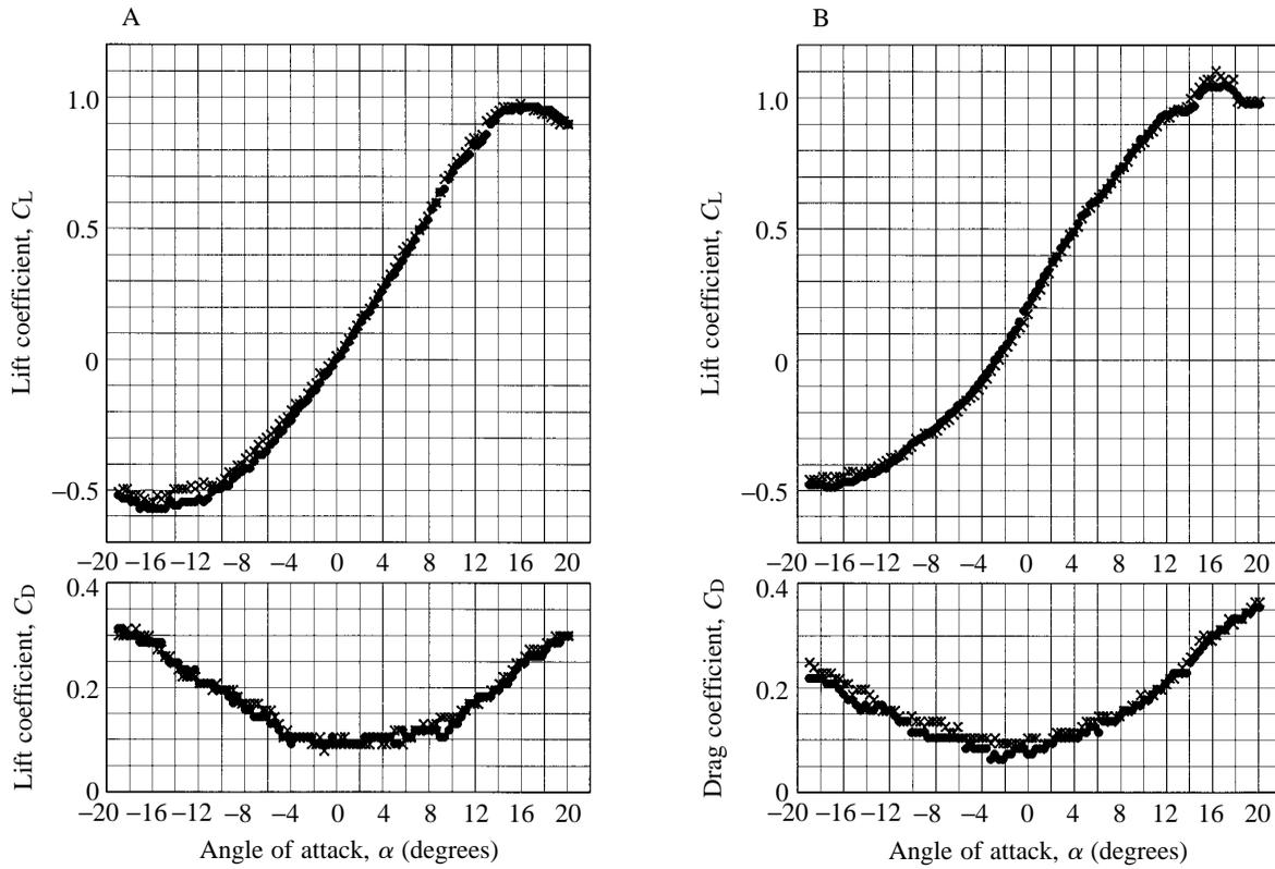
Fig. 16. Aerodynamic characteristics of the modified dragonfly wing shown in Fig. 15B. The wing pair was from dragonfly B in Table 1. Circles indicate results from tests with  $\dot{\alpha} > 0$ , where  $\dot{\alpha}$  is the rate of change of the angle of attack. Crosses are for  $\dot{\alpha} < 0$ . (A)  $C_L$  (upper panel) and  $C_D$  (lower panel) versus  $\alpha$  for the forewing ( $AR=5.9$ ). (B) Results for the hindwing ( $AR=4.5$ ).
