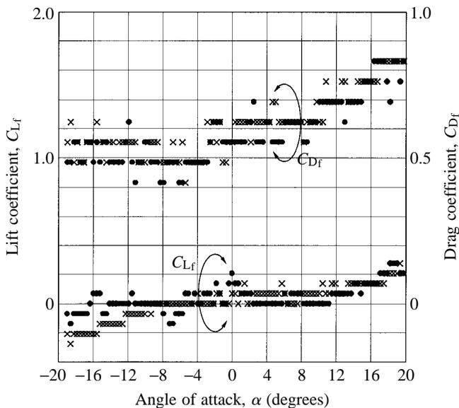
Fig. 19. The aerodynamic characteristics of the body of dragonfly A in Table 1. Filled circles represent values for which the rate of change of the angle of attack ( $\dot{\alpha}$ ) during experiments was greater than 0, crosses represent  $\dot{\alpha} < 0$ .  $Re = 2.4 \times 10^4$ .
