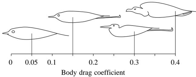
Fig. 8. Suggested values for the body drag coefficient  $C_{Db}$  for use in computer programs such as those of Pennycuik (1989) for calculating flight performance.  $C_{Db}$  may be as low as 0.05 in species whose heads and feet can be fully faired by feathers. At the other extreme, species with prominent heads and long legs may behave like 'bluff bodies' with drag coefficients as high as 0.4. These suggestions are provisional, pending actual measurements.
