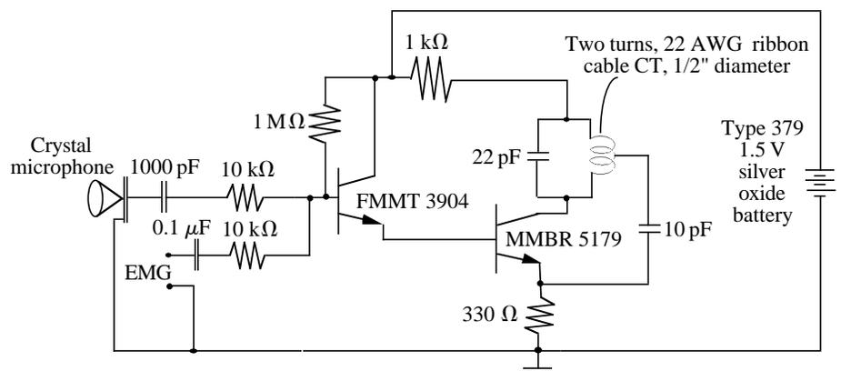
Fig. 1. Diagram of the FM transmitter.
