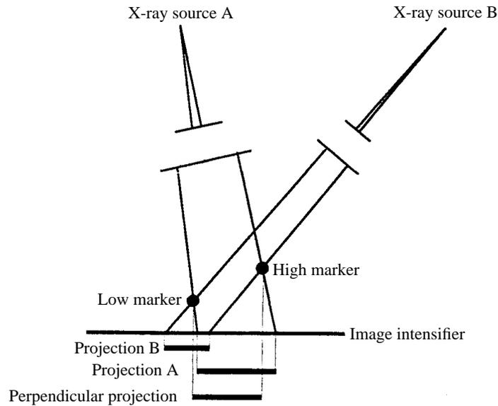
Fig. 11. Projection errors may occur when two markers have a different vertical distance from the image intensifier, as shown here. The projected distance between these markers depends on their position with respect to the X-ray source, as illustrated here for two very different positions (exaggerated) of the X-ray source (A, B) with respect to the markers.
