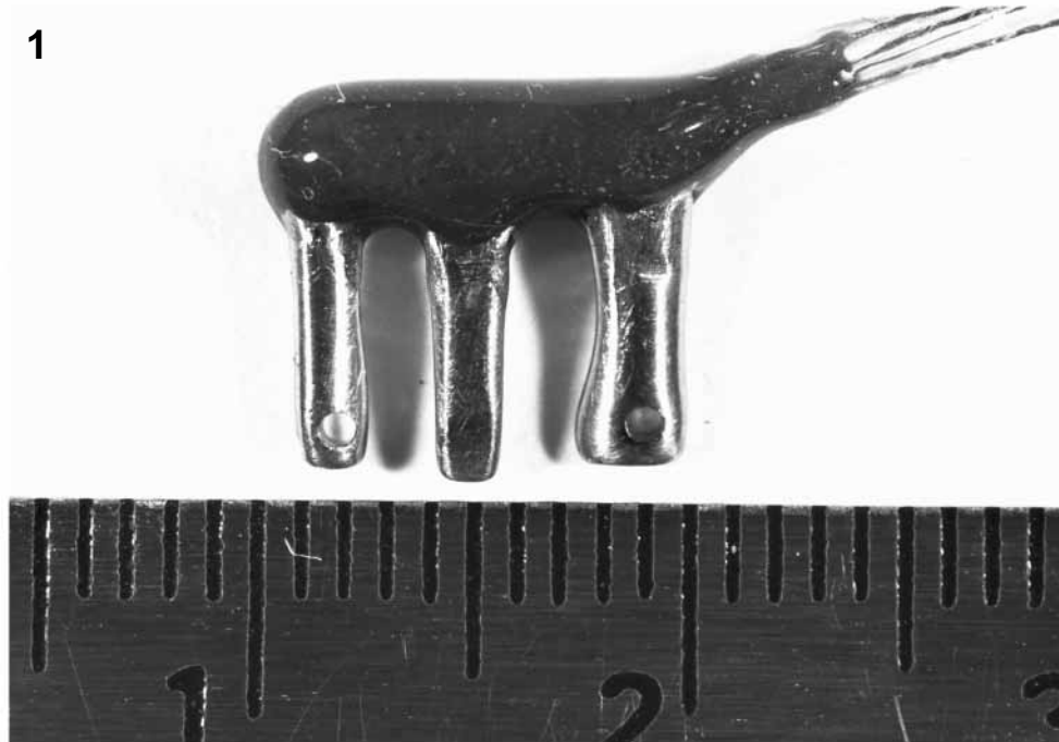
Fig. 1. Tendon transducer used for the recording of forces from cat soleus (small units on the scale shown are 1 mm). The holes at the end of the top and bottom bar of the E-shaped transducer are for suturing the transducer in place.
