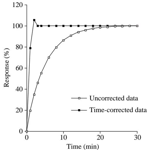
Fig. 1. Accuracy of the time resolution for the calorimetry signal. At time zero, the internal calibration heater generated a  $100 \mu\text{W}$ , square-wave signal. Values are means  $\pm 1$  s.d. ( $N=8$ ). No error bars are given because the standard deviation was within the size of the symbol.
