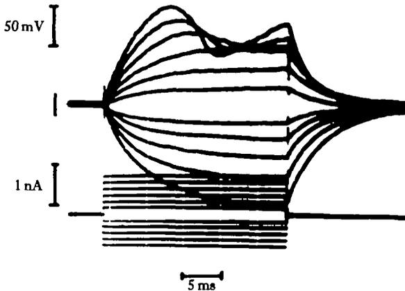
Fig. 2. Time-dependent resistance obtained during large positive pulses in the presence of  $10^{-4}\text{ M}$ -amiloride. Notice that even before reaching the time-dependent responses, the voltage deflections produced by the pulses of current were asymmetric. (From Stefani & Cereijido, 1983.)
