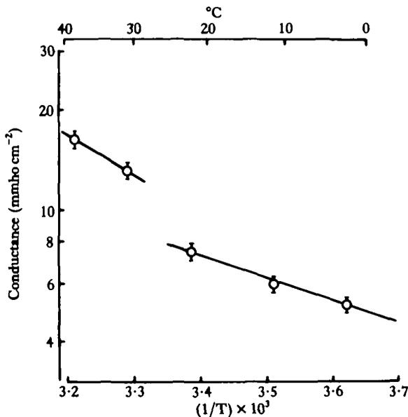
Fig. 3. Arrhenius plot of electrical conductance across monolayers of MDCK cells. Conductance was calculated with the voltage deflection elicited by a current pulse of a  $100 \mu\text{A cm}^{-2}$ . (From L. González-Mariscal, B. Chávez de Ramírez & M. Cereijido, unpublished observations.)
