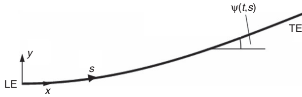
Fig. 1. Schematic flexible plate model swimmer. s is the curve length and \Psi(t,s) is the tangential angle. LE, leading edge ( s=-1 ); TE, trailing edge ( s=1 ).
