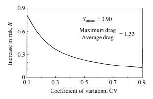
Fig. 9. Increase in risk, R, as a function of the coefficient of variation of strength for  $S_{\text{mean}}=0.90$  and  $S_{\text{max}}/S_{\text{mean}}=1.33$ . For small coefficients of variation, the increase in risk is large relative to the increase in drag.
