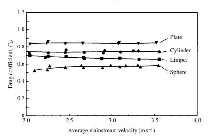
Fig. 2. Drag coefficient as a function of velocity for the objects used in this study. Within a wide range of average mainstream velocities, there is no significant variation in drag coefficient. Solid lines are third-order polynomial regressions for the entire data set for each object.
