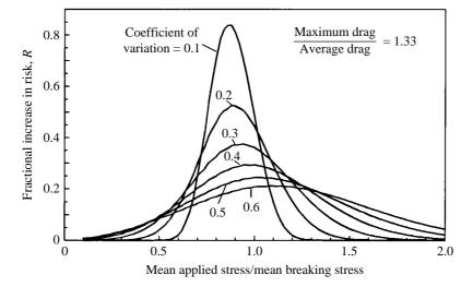
Fig. 8. The imposition of a maximal drag results in an increase in the risk of dislodgment R above that predicted for the imposition of the mean drag. The magnitude of this increase is shown as a function of the ratio of mean drag-imposed stress to the population mean breaking stress,  $S_{\text{mean}}$ .
