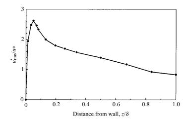
Fig. 6. The average fluctuation in velocity parallel to the wall  $(u'_{rms})$  is a function of distance from the wall. Data calculated from information presented in Figs 18.3 and 18.4 in Schlichting (1979), taken in turn from Reichardt (1938).
