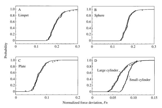
Fig. 4. Cumulative probability curves for the extreme drag forces measured on the experimental objects. Solid lines are estimates of the asymptotic probability distributions (calculated using equation 8). Note that the scale of the abscissa varies among plots.
