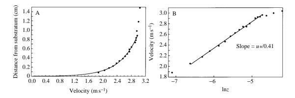
Fig. 1. The boundary-layer profile characteristic of these experiments. (A) The profile itself. The solid curve is a logarithmic fit to the 16 data points taken closest to the wall. (B) The data from A logarithmically transformed. The slope of the solid regression line is equal to the friction velocity  $(u^*)$  divided by von Kármán's constant, 0.41.
