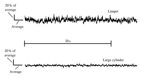
Fig. 3. Representative recordings of drag for the objects with the smallest variation (the large cylinder) and the largest variation (the limpet). The vertical scale shows 20% of the average drag recorded for the two objects, and the horizontal line marked 'average' is drawn at the level of the average force.
