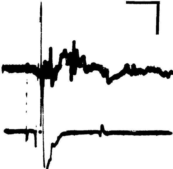
Fig. 8. Evoked potentials recorded at the base of an antenna (upper trace) and at  $N_5$  (lower trace) to stimulation at  $A_5$ - $A_4$ . First response from the antenna is marked by a dot. Note that the responses at  $N_5$  and at the antenna appear with the same delay. Calibration:  $1 \text{ mV}$ .,  $10 \text{ msec}$ .
