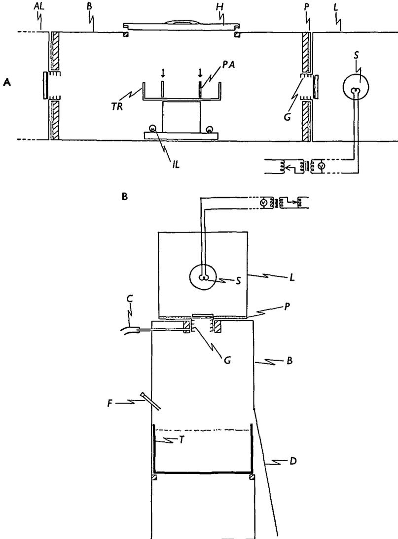
Fig. 1. (A) Phototaxis apparatus in vertical section. (B) Feeding apparatus in vertical section. *AL*, light housing (alternative position); *B* experimental box; *C*, air supply to cool filters; *D*, door; *F*, food tube; *G*, grooves for filters; *H*, hatch; *IL*, illumination used for counting larvae; *L*, light housing; *P*, foam plastic light-proofing material; *PA*, partition; *S*, light source; *T*, tank; *TR*, trough.
