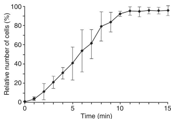
Fig. 1. Aggregation of microstome *Tetrahymena vorax* cells close to a point source of L-cysteine as a function of time. The ordinate shows the relative number of cells within the observation area (3% of the chamber surface area) surrounding the tip of a leakage pipette containing 20 mmol l<sup>-1</sup> L-cysteine in registration solution. Data are means ± s.d.
