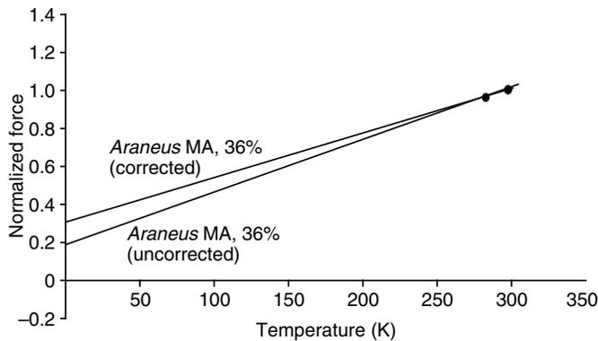
Fig. 7. A plot of normalized force against temperature for a sample of *Araneus* MA silk held at an extension of 36%. The intercept of the uncorrected plot is 0.2, indicating that for this sample approximately 20% of the force is due to enthalpy. When corrected for the effects of thermal swelling, the slope of the force–temperature plot decreases, and the intercept rises to 0.30 for this silk sample, indicating that approximately 30% of the force is due to bond energy.
