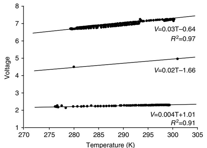
Fig. 2. The raw data from a typical thermoelastic experiment on *Araneus* MA silk. The top curve represents the raw force-temperature data and the bottom curve represents the control data for the expansion of the apparatus. A linear regression fitted to the control data was subtracted from the regression of the raw data to give the corrected voltage-temperature profile of the silk (middle curve).
