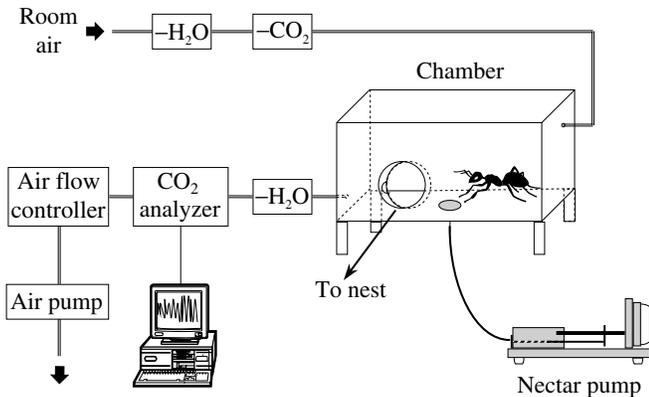
Fig. 1. Experimental design used to measure the metabolic rates of worker ants while foraging. Briefly, H<sub>2</sub>O- and CO<sub>2</sub>-free air was drawn through the respirometric chamber at a flow rate of 300 ml min<sup>-1</sup> STP. The CO<sub>2</sub> produced by the ant was measured by an IR CO<sub>2</sub> analyzer and the data were stored in the computer.
