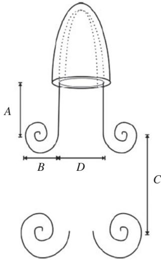
Fig. 1. Schematic of a jetting medusa with vortex rings in the wake. Vortex rings are shown in cross section. A, jet length; B, vortex ring core diameter; C, vortex ring spacing; D, jet diameter.
