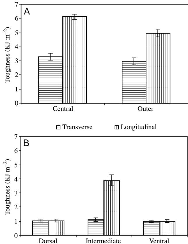
Fig. 3. Results of the cutting tests on nail clippings (A) giving the mean toughness ( $\pm$  S.D.,  $N=15$ ) of central and outer sections of the nail, when cut in the longitudinal and transverse directions and (B) showing the mean toughness ( $\pm$  S.D.,  $N=10$ ) of each of the three layers of the fingernail, when cut in the longitudinal and transverse directions.
