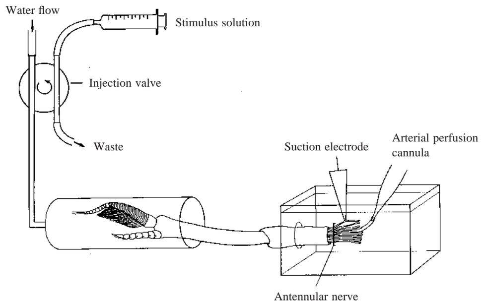
Fig. 1. Schematic diagram of the recording chamber/olfactometer used in monitoring the extracellular activity of olfactory receptor cells in blue crab (*Callinectes sapidus*) antennules.
