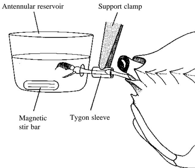
Fig. 2. Schematic diagram of the apparatus used to examine tracer flux between the hemolymph and the sensillar lymph, and to measure trans-antennule potential. The crab (shown to the right) was secured to a stable platform and remained out of water during the course of an experiment.
