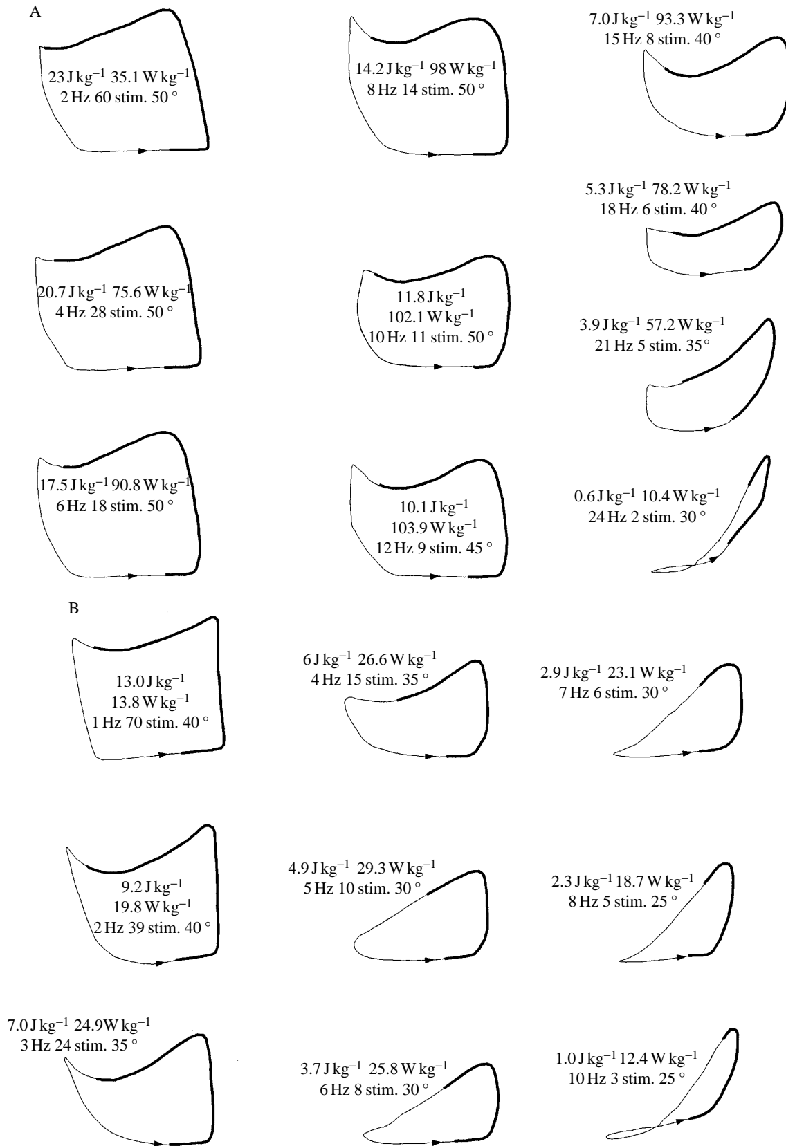
Fig. 1. The effects of cycle frequency on (A) EDL and (B) soleus work loop shape, using constant \pm 5\%L_0 strain amplitude under conditions for maximal power output. The period of stimulation is shown by the thickened line on each work loop. In each cycle, the work done and the mean power output of all muscles studied are shown. Also given are cycle frequency, number of stimuli and phase shift (in degrees). Arrow shows direction of loop.
