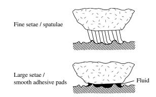
Fig. 4. Schematic diagram illustrating two possible strategies of compensating small-scale surface roughness (roughness smaller than the dimensions of the pad). Good adhesive contact can either be achieved 'dry' with very fine seta tips or 'wet' by secretion of a fluid that can fill out substrate cavities. A fluid may not only be necessary in smooth adhesive pads (e.g. many insects and tree frogs) as shown here but also in hairy pads, when setae are relatively large and blunt as in many insects.
